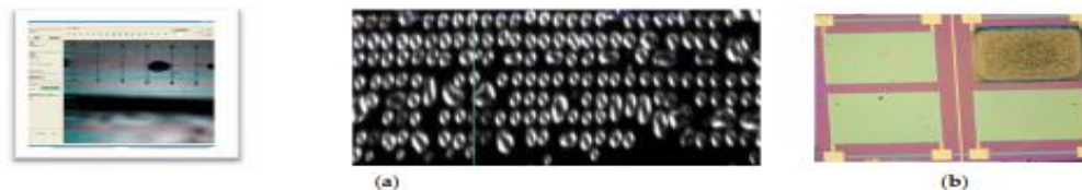
Figure 15. (a) Images during the printing process of the PANI:PSS/SWCNT ink with Dimatix DMP 2800; (b) Optical microscope image of PANI:PSS/SWCNT on one pair of IDEs.
