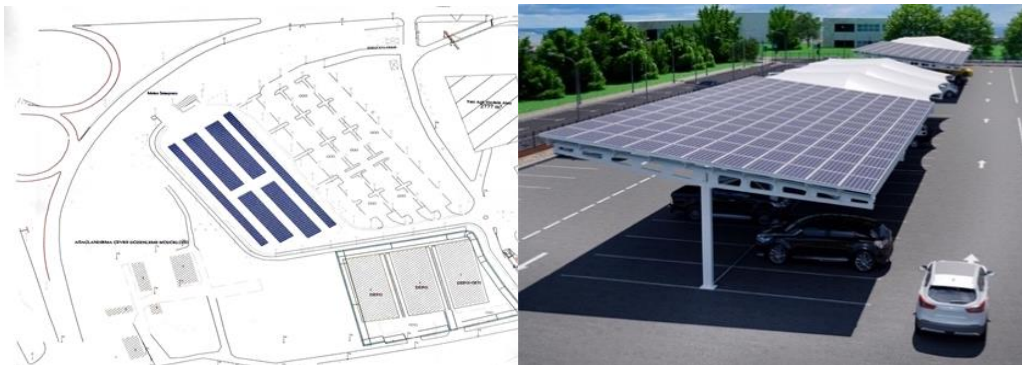
Fig -3: 600 kW grid-connected car-park PV system with electric car chargers (to be completed in 2022)
