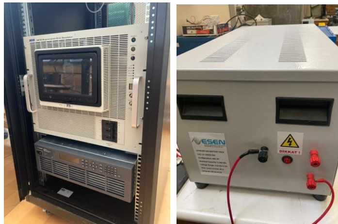
Fig -2: 1000V, 60A PV Simulator, 12 kVA Grid Simulator, Lithium Ion Battery Pack (3x2.25kWh, 30A)
